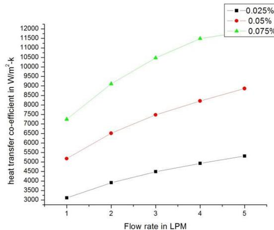
**Fig 3.3** heat transfer co-efficient vs. flow rate
