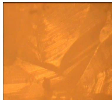
Figures: 14-19 shows the corroded metal surface of Al, Cu, MS coupons in 0.5 N and 2.0 N HCl acid solutions
