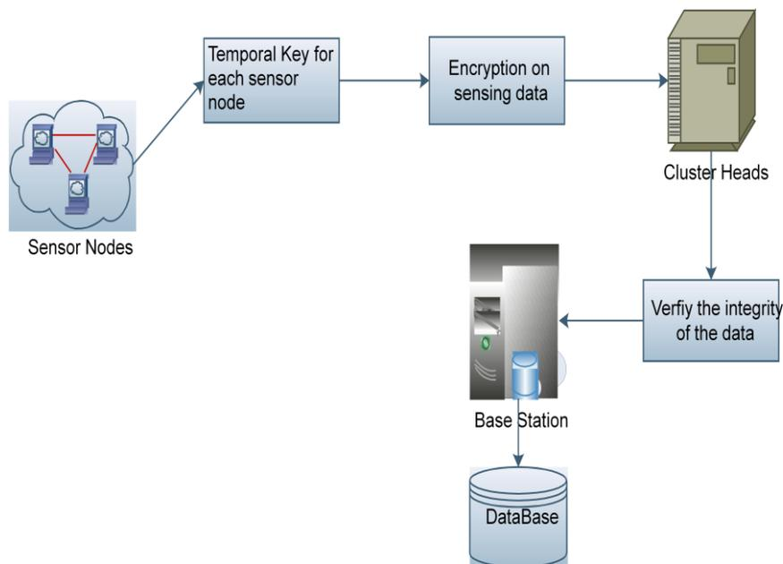
Fig 1 The proposed framework for Data Integrity analysis in wireless sensor networks
