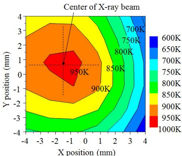
**Figure 5.** The measured temperature distribution on the a-Si film/glass substrate. The storage-ring current and undulator gap were 220 mA and 46.7 mm (photon energy of 115 eV). The measurement points were 9 points by each 4 mm length.
