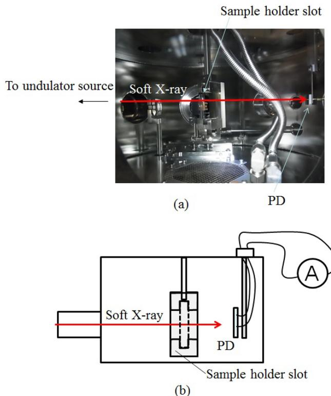
**Figure 2.** (a) Optical image of the inside of soft X-ray irradiation chamber. (b) Setup for measuring the photocurrent.
