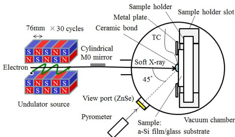
**Figure 1.** Schematic diagram of soft X-ray irradiation. Setup for measuring the sample temperature using a TC and a pyrometer was also shown. The soft X-ray generated at the undulator source irradiated with the sample surface via MO mirror.
