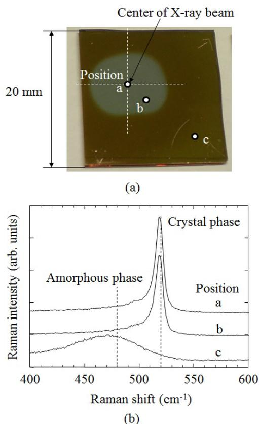
**Figure 7.** (a) Optical image of the soft-X-ray-irradiated a-Si film/glass substrate. (b) Raman spectra measured at positions a, b, and c.
