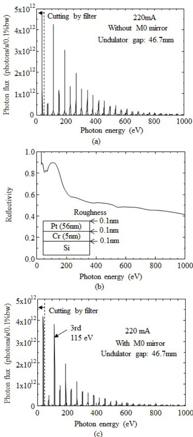
**Figure 4.** (a) Calculated photon flux at the undulator gap of 46.7 mm and the storage-ring current of 220 mA. (b) Reflectivity of MO mirror with Pt (56 nm)/Cr (5 nm)/Si substrate. The cross-sectional structure of MO mirror is illustrated in insert. (c) Photon-flux dependence of photon energy on the sample surface was calculated by product of photon flux generated from the unduator source by the reflectivity of the MO mirror.
