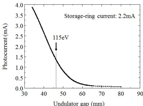
**Figure 3.** Photocurrent as a function of undulaor gap. The photocurrent was measured using the PD at the storage-ring current of 2.2 mA. The undulator gap at 115 eV was shown as an arrow.
