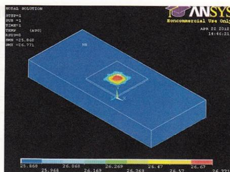
**Figure 6.** The calculated temperature distribution. (a) Calculation model. (b) Temperature distribution of a-Si/glass substrate during the soft X-ray irradiation.
