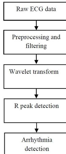
Fig 2 R-peak detection structure
