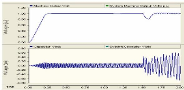
Fig.4. Oscillation at the output and capacitor voltage is increased at resistance 6.0832 Ω.
