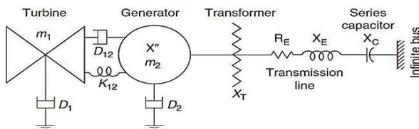
Fig.1. Turbine and generators unit of thermal is connected to series compensated system.
