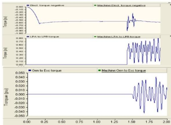
Fig.7. Oscillation at Generator to exciter torque is decreased at resistance 95Ω.
