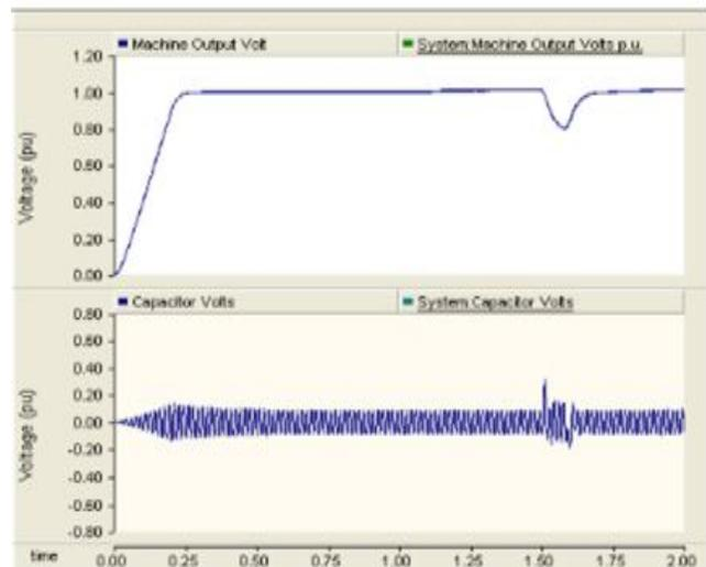
Fig.6. Oscillation at the output and capacitor voltage is decreased at resistance 95Ω.
