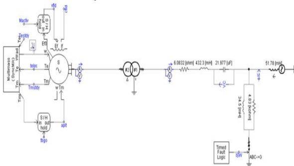
Fig.3. Simulation of thermal unit carried out for various level of series compensation
