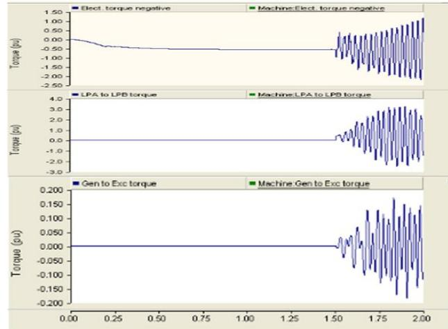
Fig.5. Oscillation at Generator to exciter torque is increased at resistance 6.0832Ω.
