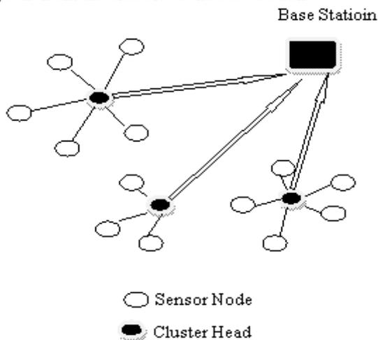
Figure 4. Graph showing construction of cluster in LEACH
