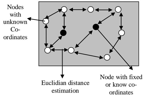
Fig 2: Setup of Greedy Algorithm
