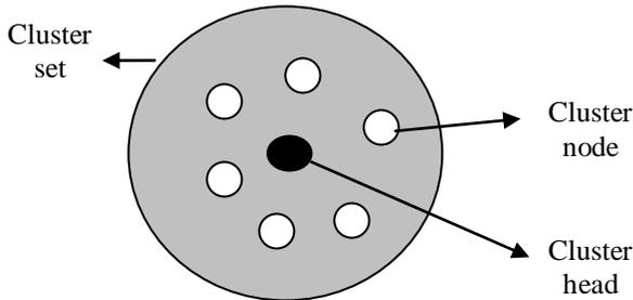
Fig 1: Setup of LEACH Algorithm
