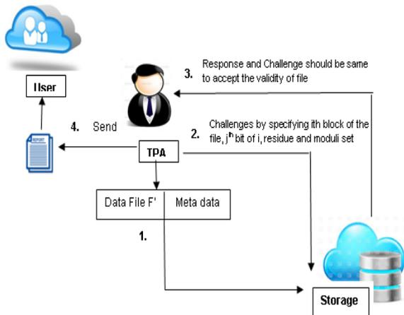
functions and calculates the MD and report to the TPA. The following figure shows the process of inspection phase.
