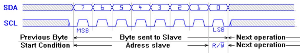
Fig 5: Transmission of a byte to a slave
