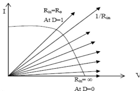
Fig 9: The range of  $R_{in}$  values for buck converters
