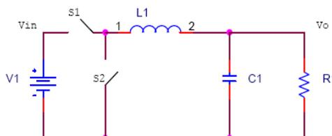
Fig 8: Buck Converter
