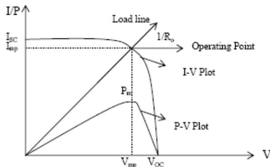
Fig 3: V-I and P-V characteristics of the PV cell
