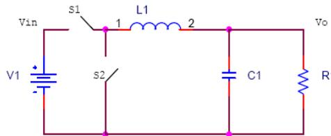
Fig 8: Buck Converter
