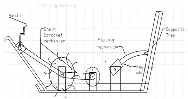
**Figure 2:** Proposed system for Planter Machine.
