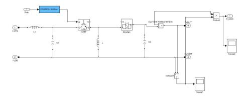
Figure 5 Matlab Model Of Buck Boost Converter.
