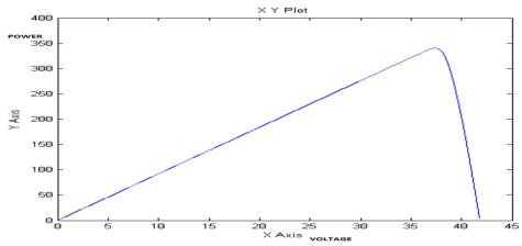
Figure 9: P-V Plot Of Solar Cells
