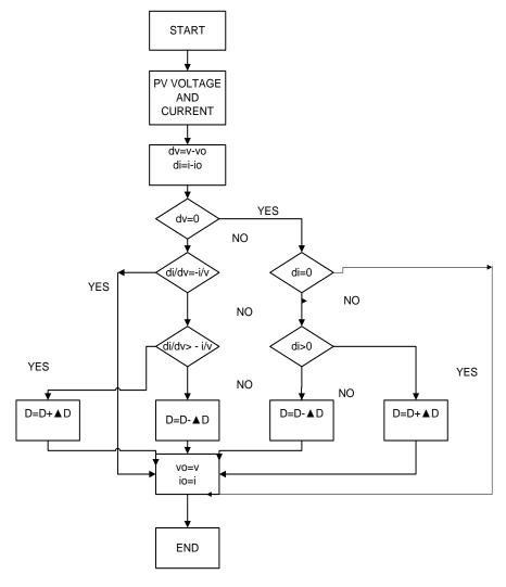
Figure 4: Flow Chart Of INC Algorithm
