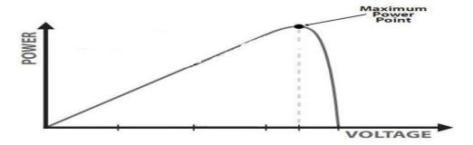
Figure 3.INC algorithm wave form
