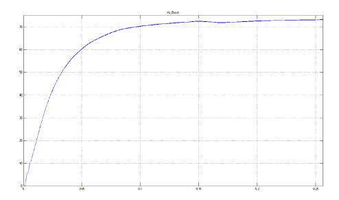
Figure 11: Voltage Output Of Buck Boost Converter
