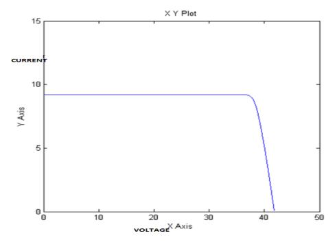
Figure 8: V-I Plot Of Solar Cells
