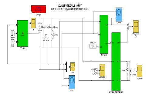
Figure 6: Simulink Model Incremental Conductance Method
