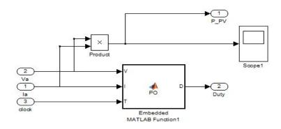
Figure 7: Matlab Embedded Function For INC Algorithm
