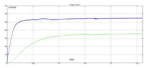
Figure 10 Power Output Of MPPT And Buck Boost Converter
