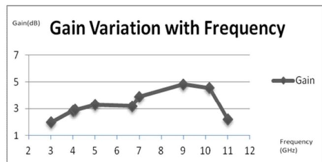
Figure 13: Variation of Gain with frequency
