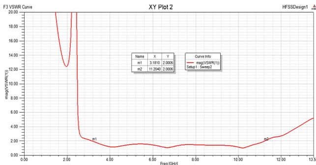
Figure 12: VSWR curve for 3FA Antenna
