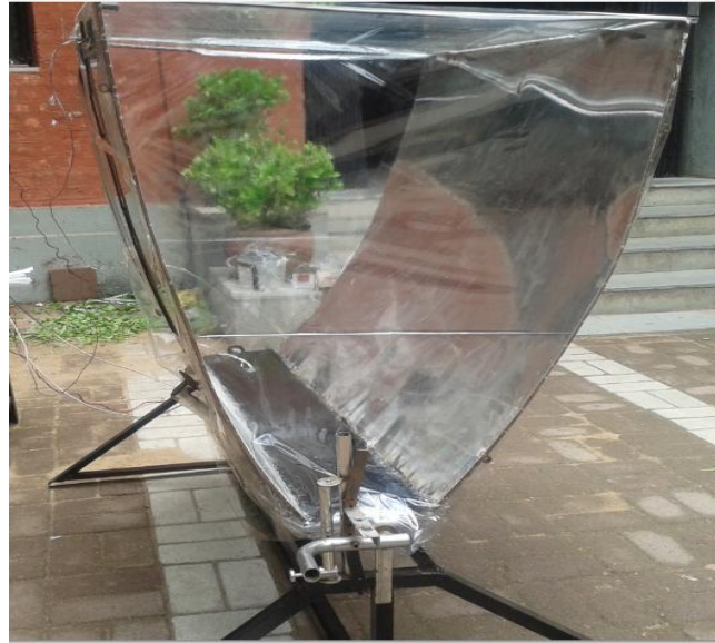
Fig:4 Fabricated 2-D Compound Parabolic Concentrator
