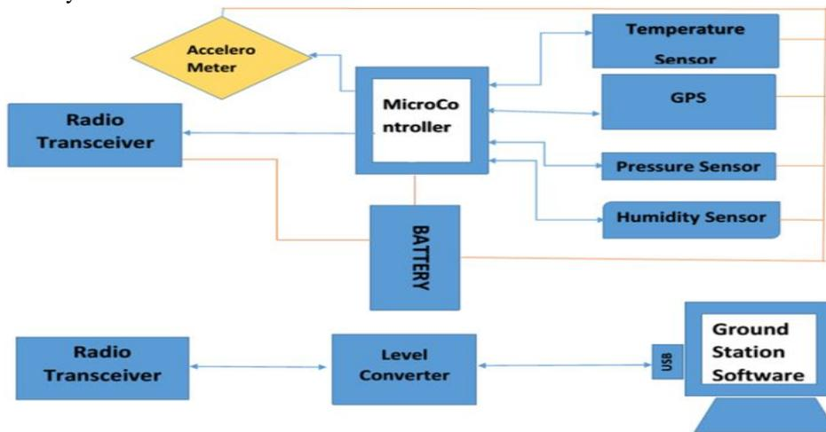
Figure2.Electrical architecture block diagram and ground station
