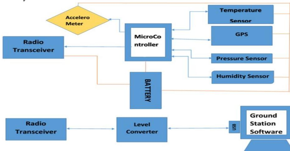
Figure2.Electrical architecture block diagram and ground station
