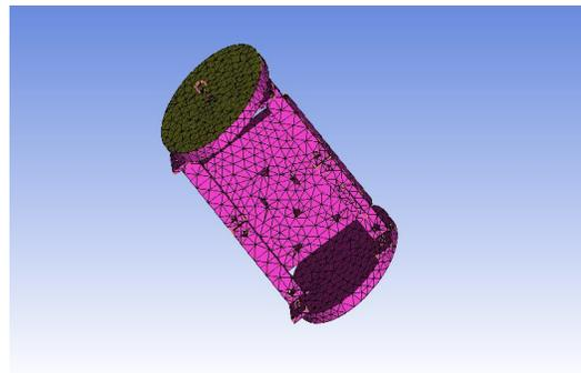
Figure5. Mesh Geometry in Ansys Software
