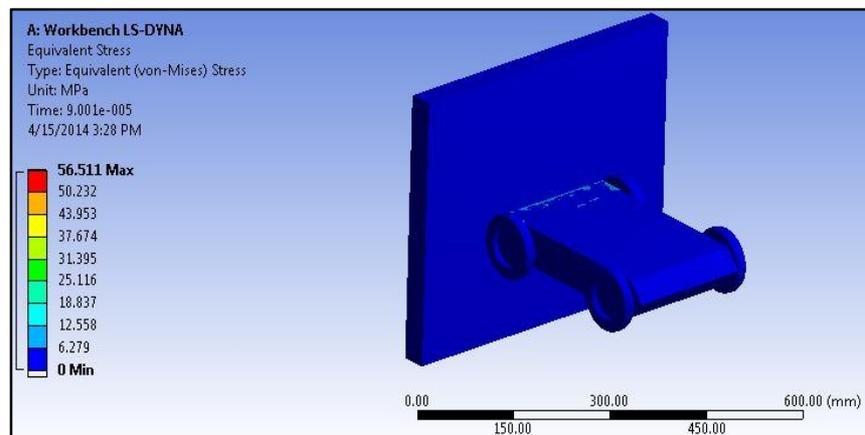
Figure 12: Von Mises stress for 3 m/s velocity
