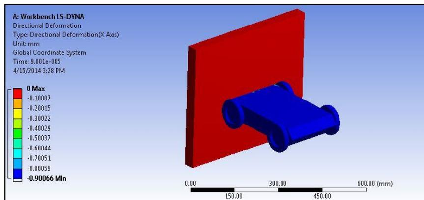
Figure 10: Directional Deformation along X – Axis
