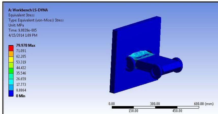
Figure 11: Von Mises stress for 10 m/s velocity
