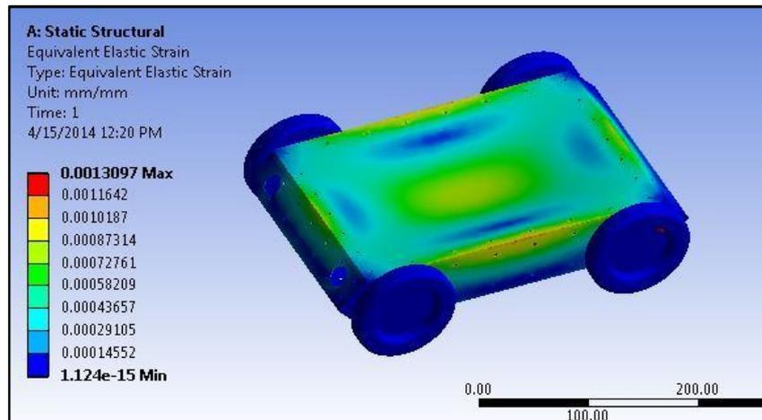
Figure 7: Elastic Strain for the Applied Load
