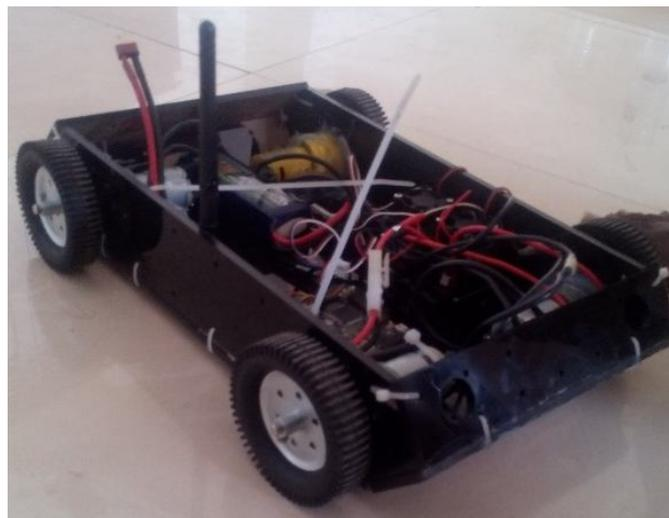
Figure 4: Fabricated model of the AGV
