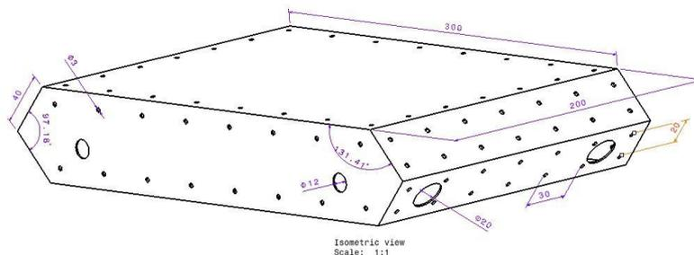
Figure 2: Isometric view of the body of UGV
