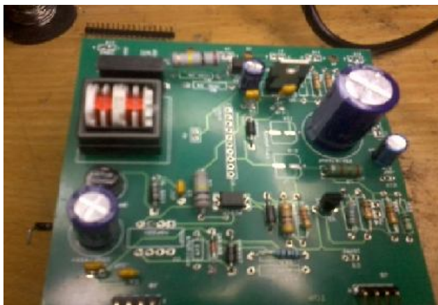
Fig.18: Component Placement of Power Supply Board
