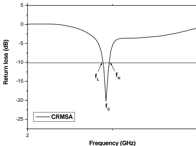
Fig. 3 Variation of return loss versus frequency of CRMSA
