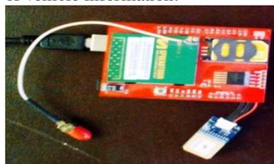
Fig. 2: The GSM/GPRS Module with the GPS Module
