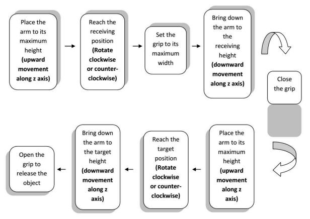
Fig. 2 Block diagram showing sequence of operations
