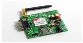
Fig.5 GSM Modem (SIM900)
