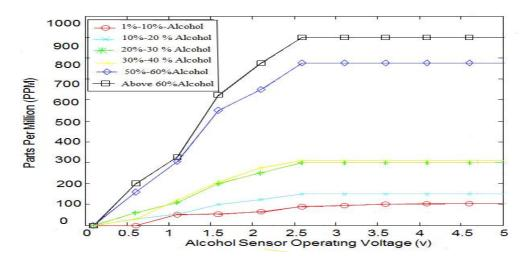
Graph 1: Response of ppm (In Percentage) via alcohol sensor output voltages values
