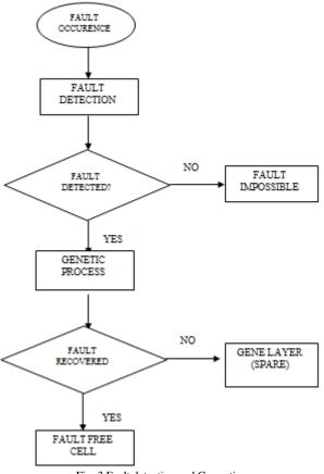
Fig .3 Fault detection and Correction
