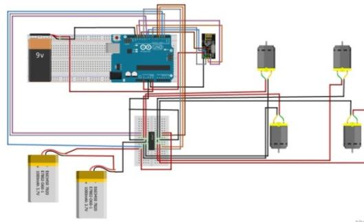
Figure 21. Breadboard implementation of a multipurpose RC vehicle with DC motor.
