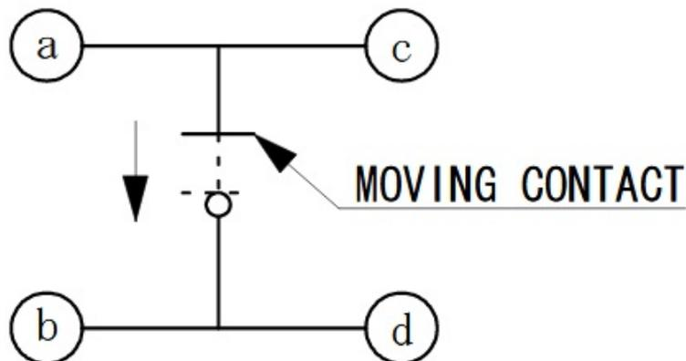
Figure 9. Schematic diagram of push button.
