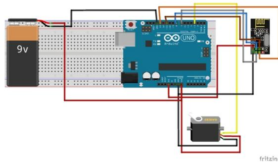
Figure 19. Breadboard implementation of a servo motor connection.
