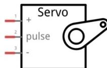
**Figure 11.** Schematic diagram and pinout of a servo motor.
