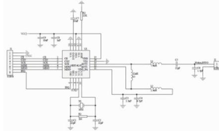
Figure 5. Schematic diagram of nRF24L01.
