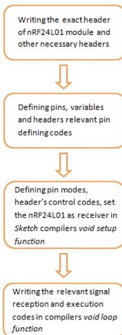
Figure 24. Programming flow chart of the receiver.
