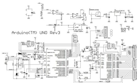
Figure 2. The schematic diagram of Arduino Uno board.
