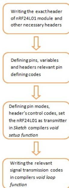
Figure 23. Programming flow chart of the transmitter.
