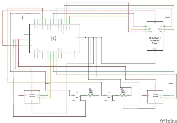
**Figure 14.** Schematic diagram of the transmitter unit.
