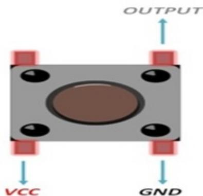
Figure 10. Pinout of the push button.
