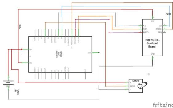
Figure 20. Schematic diagram of the servo motor control system with wireless controller.
