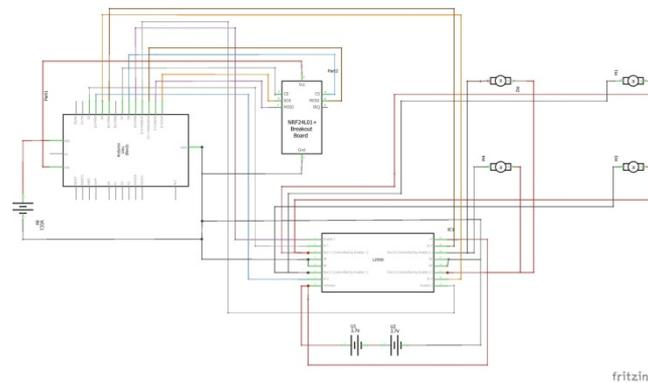
Figure 22. Schematic diagram of a multipurpose RC vehicle with DC motor.
