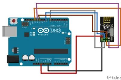
**Figure 15.** Implementation of basic receiver unit.
