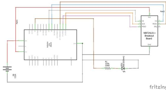
Figure 18. Schematic diagram of LED controlling.
