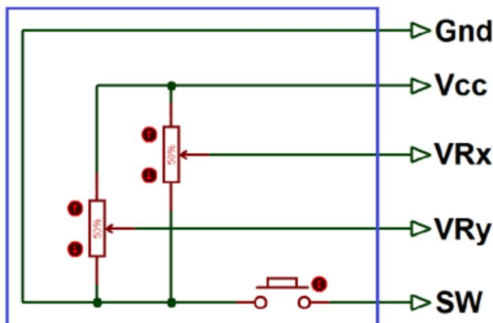
Figure 7. Schematic diagram of the joystick module.
