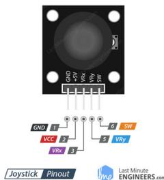
Figure 8. Pinout of joystick module.
