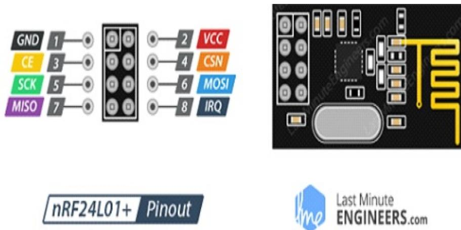
Figure 6. Pinout of nRF24L01.
