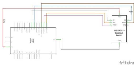
**Figure 16.** Schematic diagram of the basic receiver unit.
