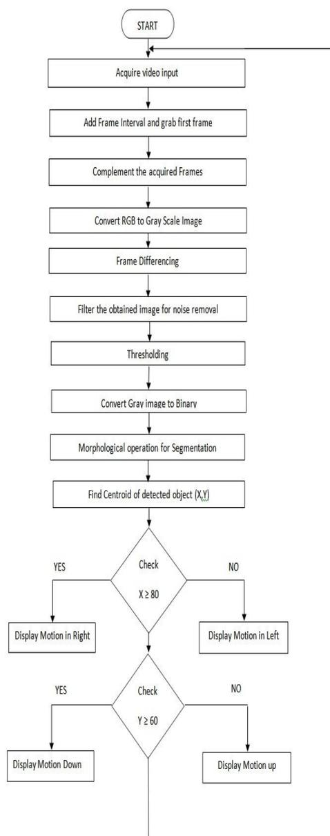
Fig. Flowchart of Object Tracking based on Yellow Color
