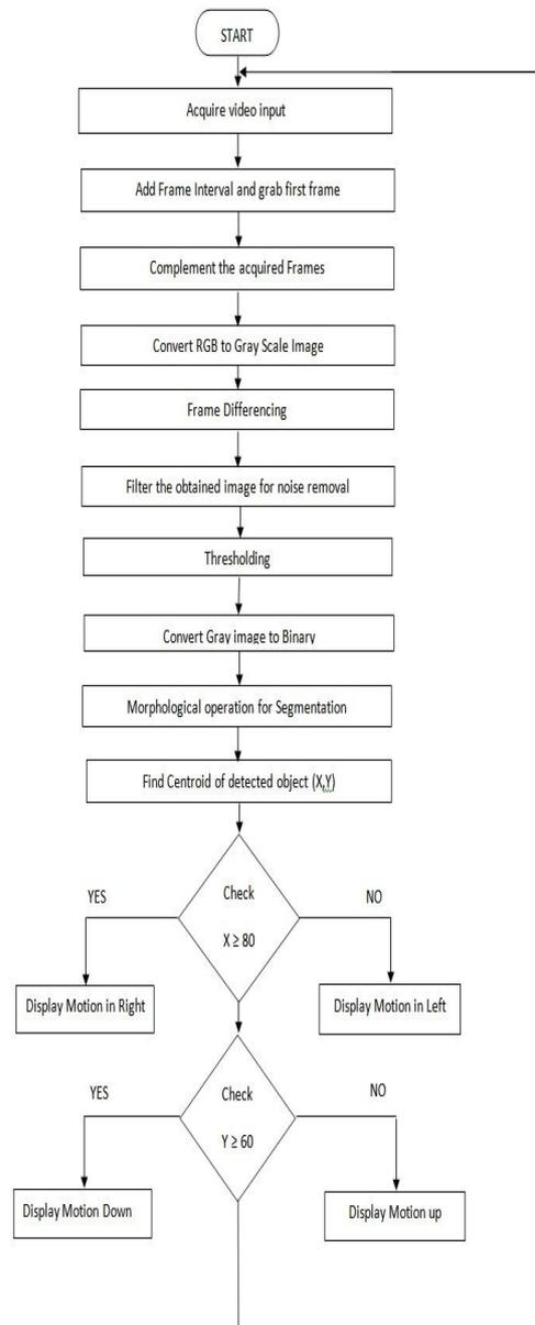
Fig. Flowchart of Object Tracking based on Yellow Color
