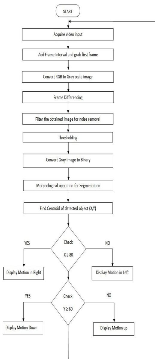
Fig.Flowchart for Human Face Tracking
