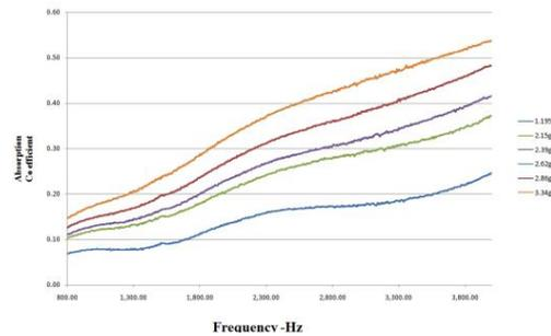
Figure 4. Absorption Coefficient of glass wool.
