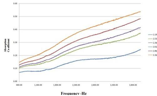
Figure 4. Absorption Coefficient of glass wool.
