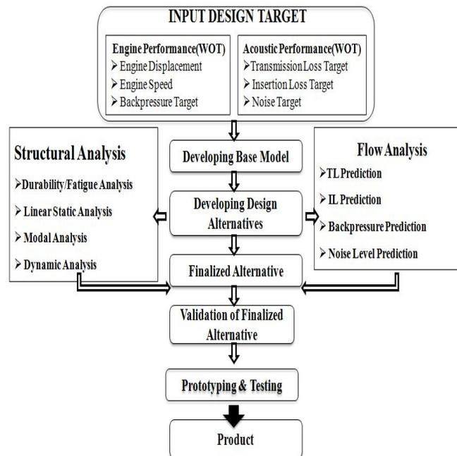
Figure 2.Muffler Design Methodology.
