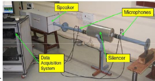
Figure 5. Experimental setup for base model.
