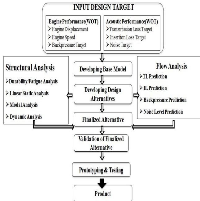
Figure 2.Muffler Design Methodology.
