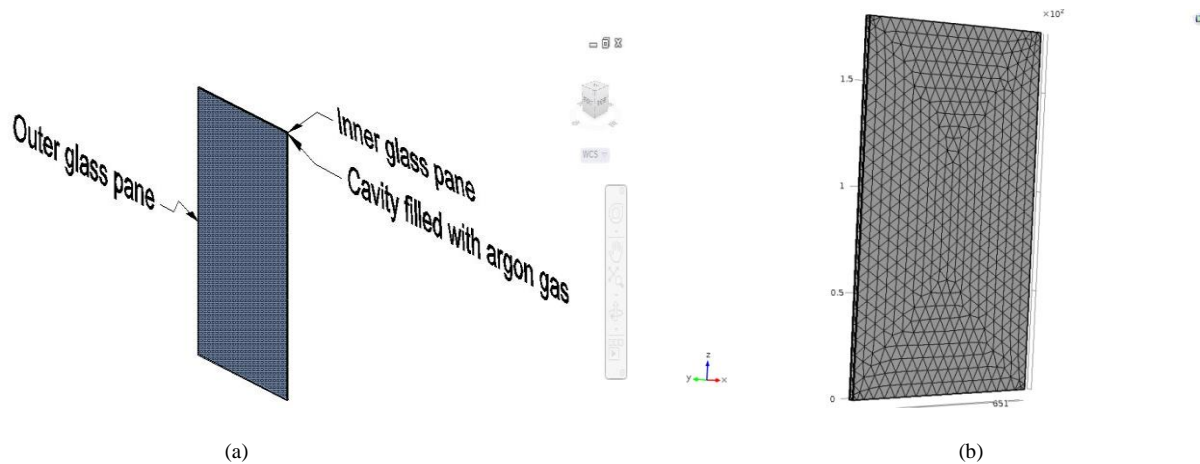
Fig. 4. Double glazing model in 3D (a) Cad model of double glazing with reflective blue coating (b) Geometry of double glazing meshed
