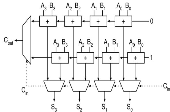
Fig 1.1 4-Bit Carry Select adder.
