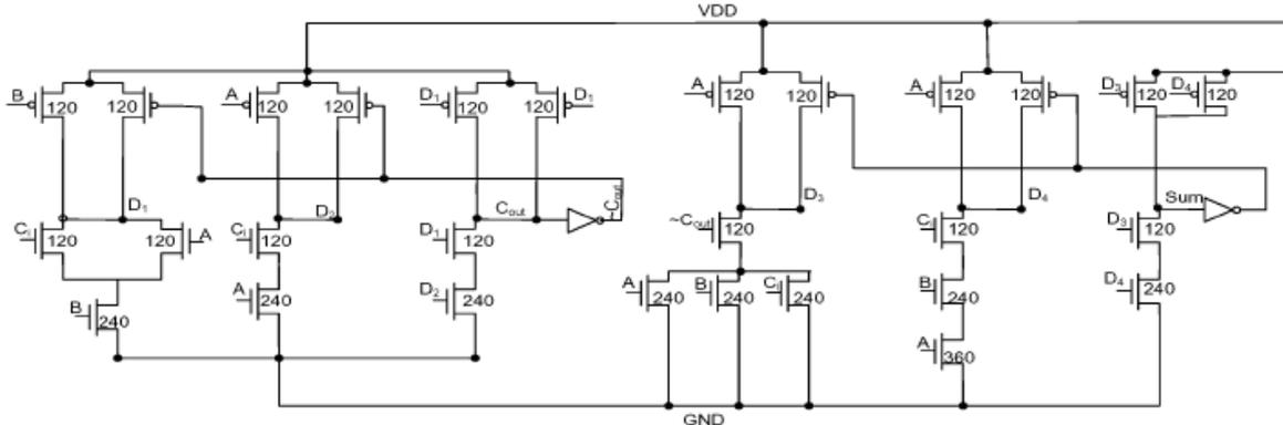
Fig.2.2 sp-D3L Logic Adder2
