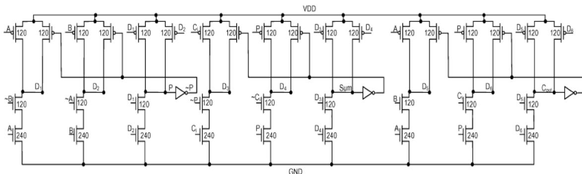
Fig.2.3 sp-D3L Logic Adder3
