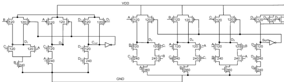
Fig.2.1 sp-D3L Logic Adder1
