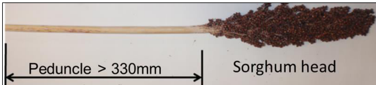
Fig. 4: Sorghum head with a peduncle attached before being mounted on the testing platform of the stripper rig
