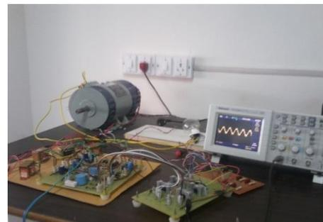
Fig. A4 Control and bridge rectifier circuits with motor load
