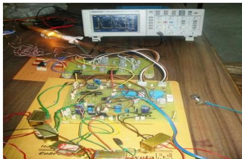
Fig. A3 Control and bridge rectifier circuits with resistive load.
