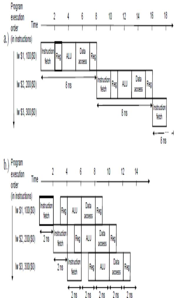
Figure 2. Single-cycle non-pipelined (a) vs. pipelined execution (b)
