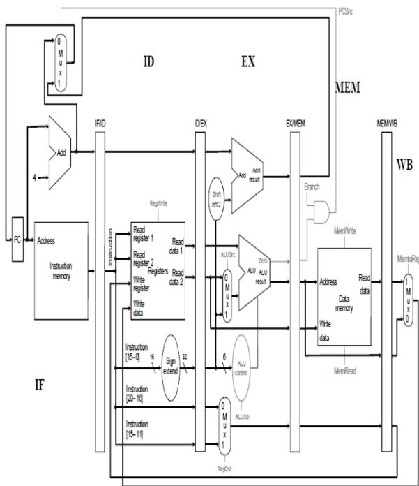
Figure 3. MIPS Pipelined Processor Datapath
