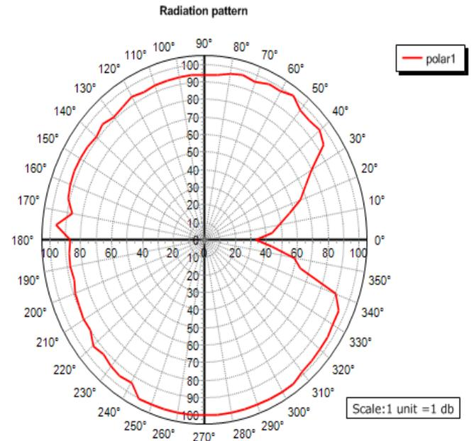
Figure 10. Radiation Pattern of Multi-Standard Patch Antenna
