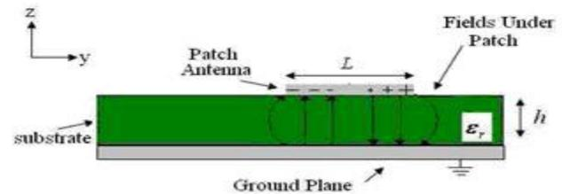
Figure 1. Microstrip Patch Antenna
