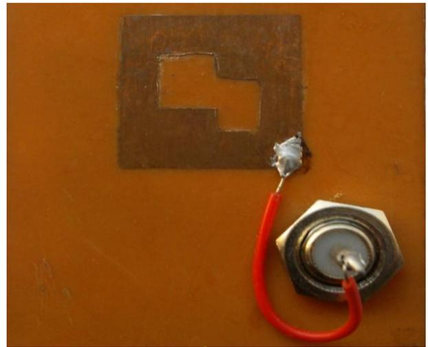
Figure 6. Circularly Polarized Microstrip Patch
