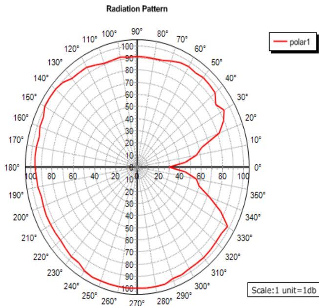
Figure 8. Radiation Pattern of E-shape patch and U-shape Patch
