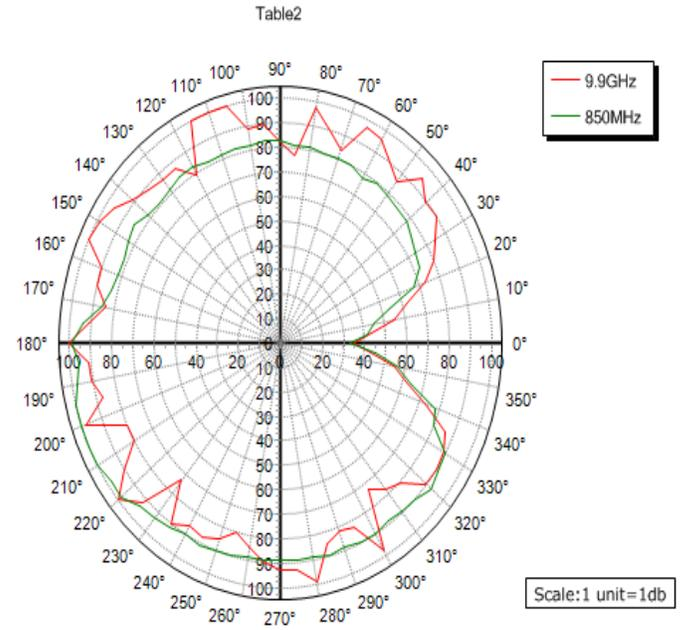
Figure 9. Radiation Pattern of Rectangular Fractal Antenna
