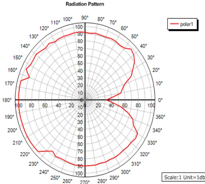
Figure 11. Radiation Pattern of Circularly Polarized Microstrip Patch
