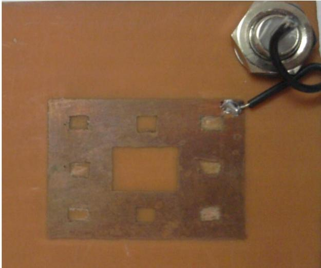
Figure 4. Rectangular Fractal Antenna
