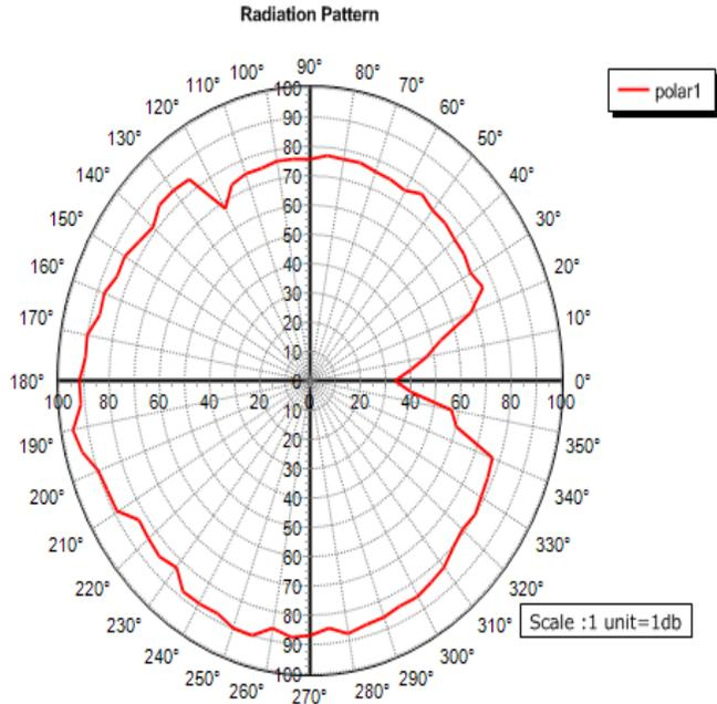
Figure 7. Radiation Pattern of Patch with two 'U'slots
