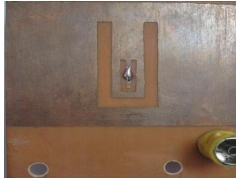
Figure 2. Patch with two ‘U’ slots
