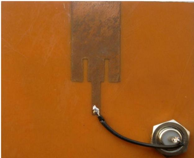
Figure 5. Multi-Standard Patch antenna
