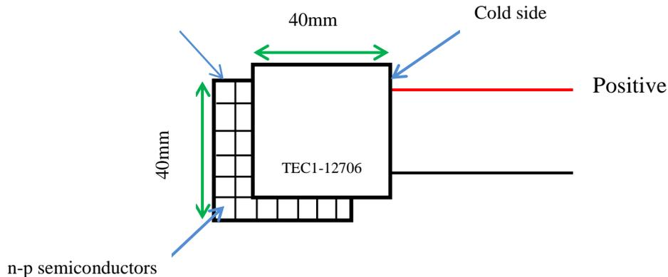
Fig. 1 Thermoelectric cooler structure
