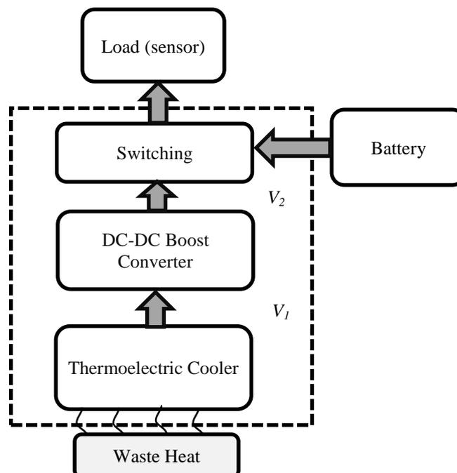
Fig. 2 Block diagram of the designed thermoelectric power source
