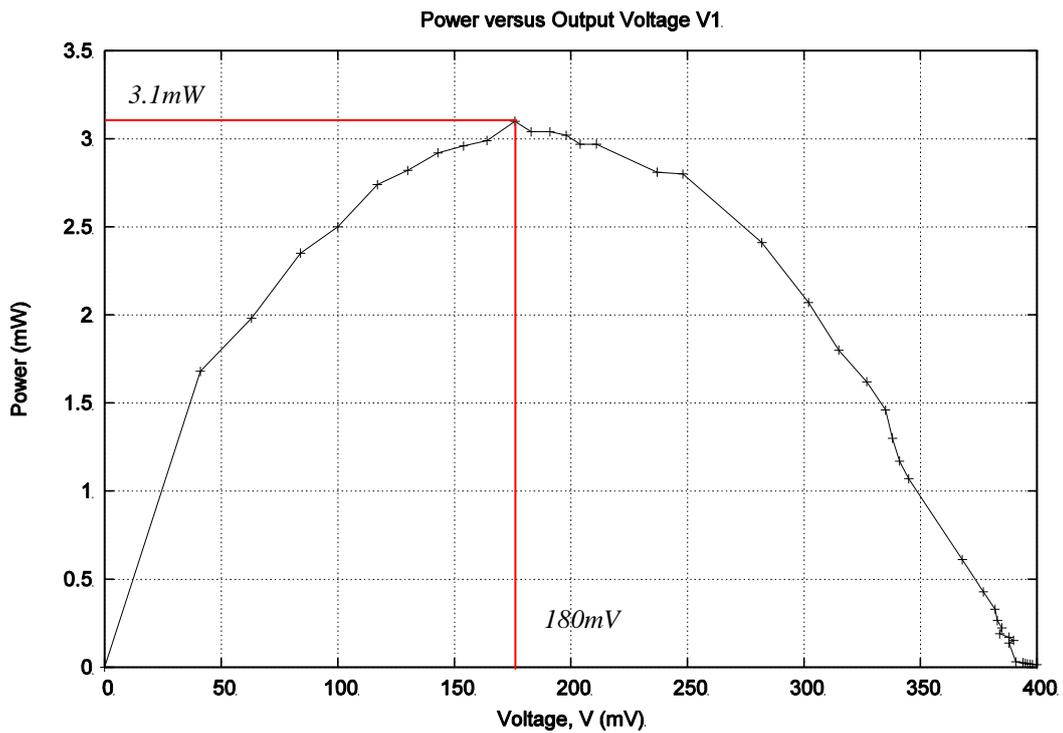
Fig. 6 Maximum power tracking of TEC
