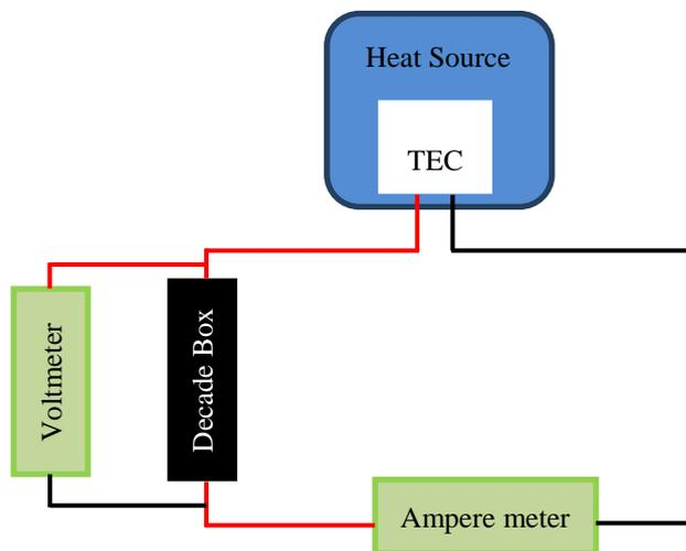
Fig. 4 Experiment circuit of TEC characterization
