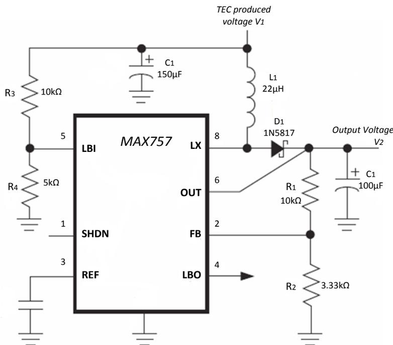
Fig. 3 Schematic circuit of the designed DC-DC Boost Converter
