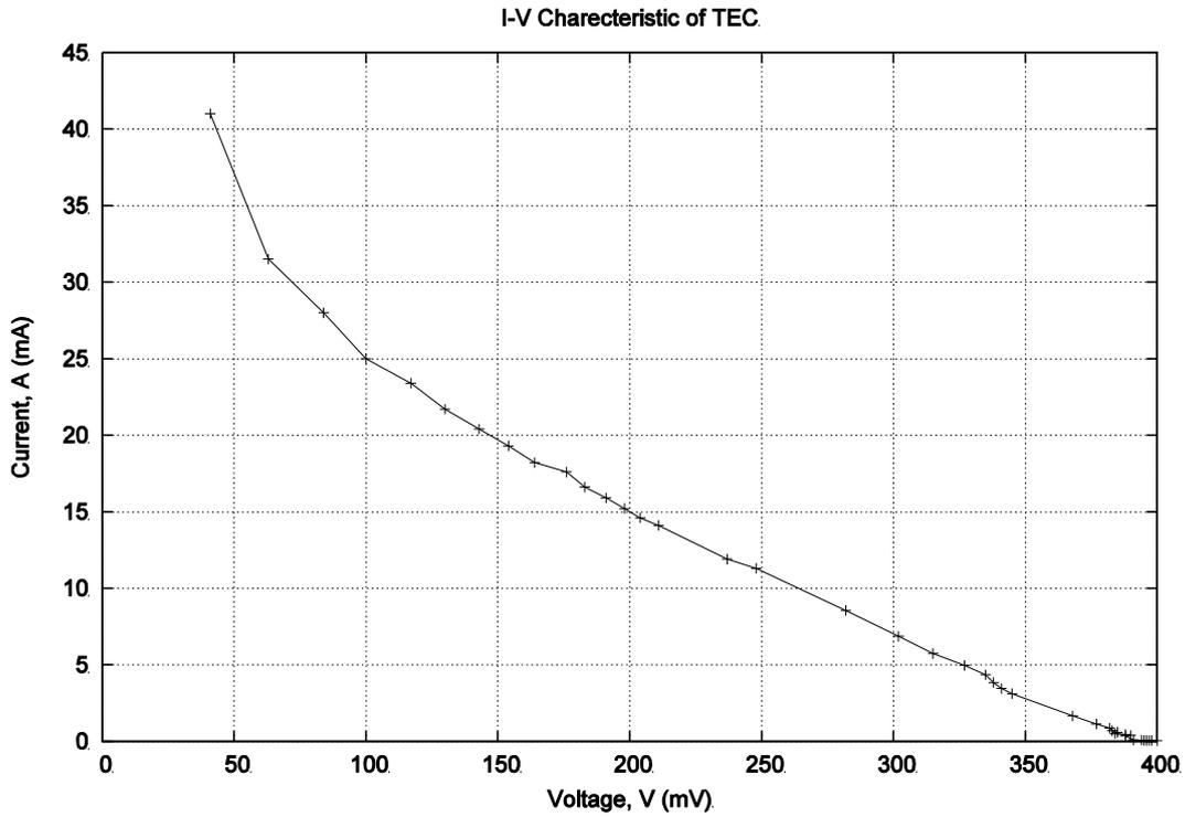
Fig. 5 Relationship between current and output voltage,  $V_1$
