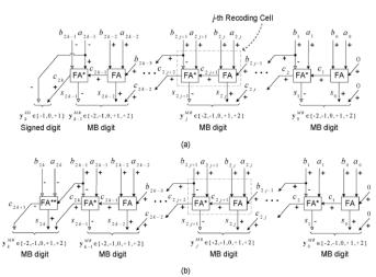
Fig.3S-MB1 recoding scheme for (a) even and (b) odd number of bits
