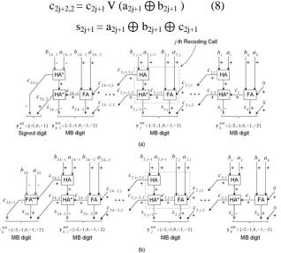
Fig.4 S-MB2 recoding scheme for (a) even and (b) odd number of bits
