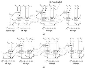
Fig.5 S-MB3 recoding scheme for (a) even and (b) odd number of bits.
