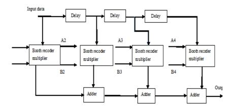
2,A3,A4----> Coefficient values 2,B3,B4----> Constant zero for addition process in smb scheme
