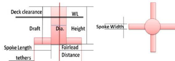
FIGURE 3. SUPPORT PARAMETERS
