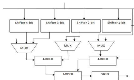
Fig. 9 Architecture of the Reconfigurable calculation Unit.
