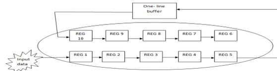
Fig. 7 Structure of ten shift registers
