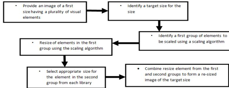
Fig. 2 Processing steps in image scaling
