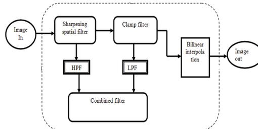
Fig. 5 shows the block diagram for the algorithm of the image scaling processor.
