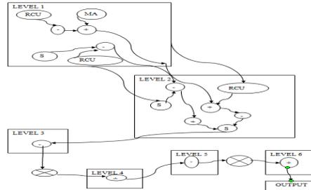
Fig. 8 Pipelined architecture for the combined filter and bilinear interpolator.
