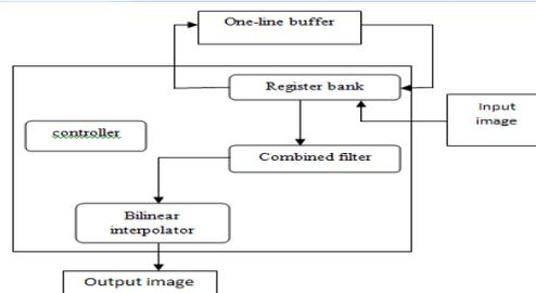
Fig. 6 VLSI Architecture
