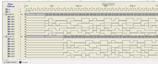
Fig.11 Simulation waveform for the register bank
