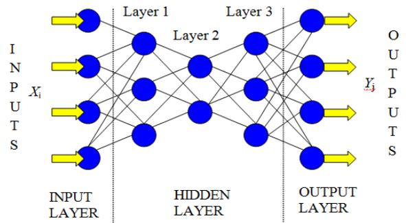
Figure 2: Generalized Structure of Multi Layer Perceptron (MLP) Neural Network Model
