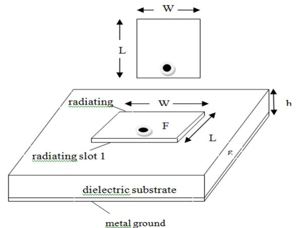
Figure 1: Rectangular microstrip antenna
