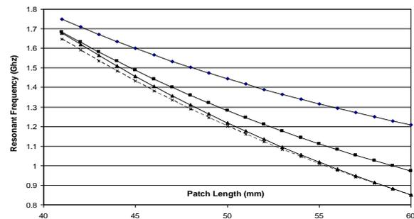
Figure: 6 Variation of Resonant frequencies with patch length.
