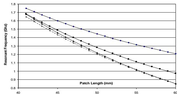
Figure: 6 Variation of Resonant frequencies with patch length.
