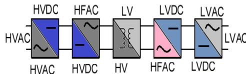
The three stage topology offers some advantages over the other two, such as [1]; reduced size due to a high frequency transformer, power factor improvement is possible, multi-level converter topologies can be applied to get high voltage levels (e.g., 11 and 22 kV). It is the three stage topology which is most prevalent now and various potentials of the power electronic circuit involved, like reduced switch topology, are being studied and developed for better proficiency.
