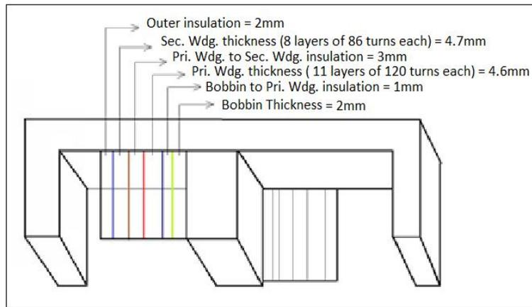
Fig 2 Winding arrangement of 200 VA, 50 Hz
