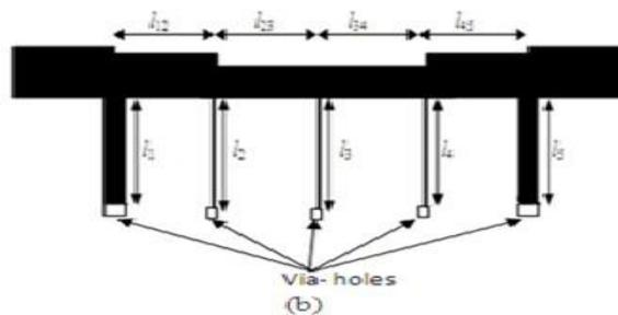
Fig1.4(a) Designed Ultra Wide Bandpass filter using quarter wave short circuited stubs (b) layout of ultrawide bandpass filter
