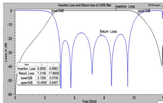
I. Fig1.5: simulated result (a) S11 (dB) and S21 (dB) (b) phase response
