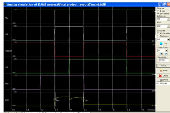
5.1 Simulation of 7-T NOR-type MCAM Cell and 7-T NAND-type MCAM Cell
