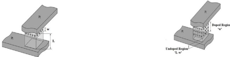
(a) "OFF" state, high resistance (b) "ON" state, low resistance Fig.1. Memristor switching behaviour
