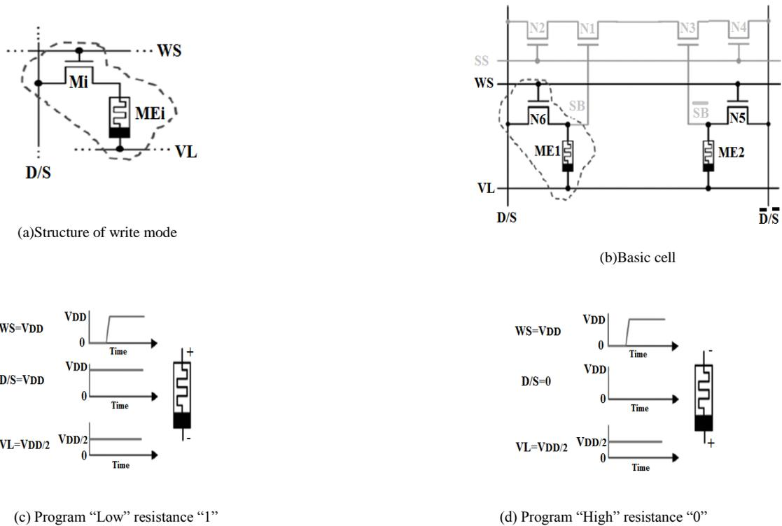
Fig.2. Basic memristor-nMOS storage cell and the timing diagram
