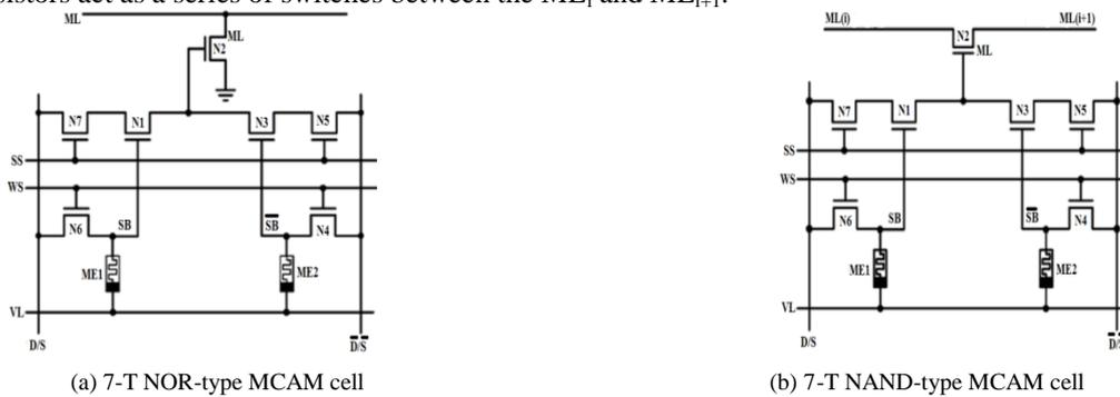
Fig.3.1 Cell configurations of possible MCAM structure
