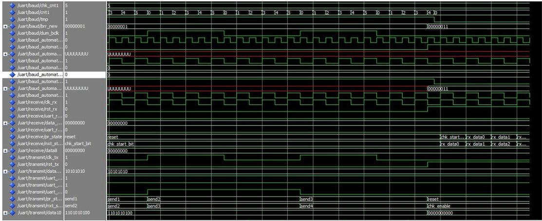
Fig 7 simulation result of automatic baudrate detection
