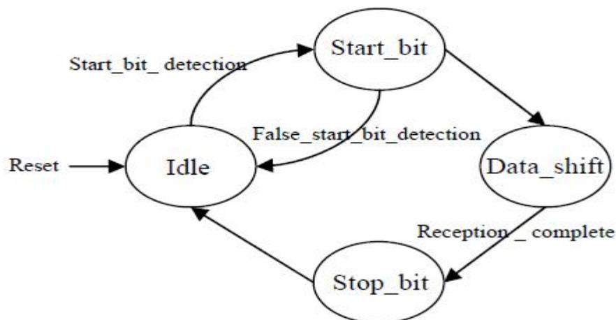
Figure 4 State diagram of a receiver unit.
