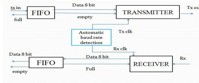
Fig1:Basic block diagram of UART.
