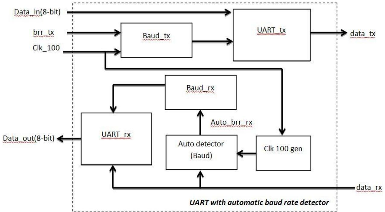
Fig 6 Complete architecture with automatic baud rate detector
