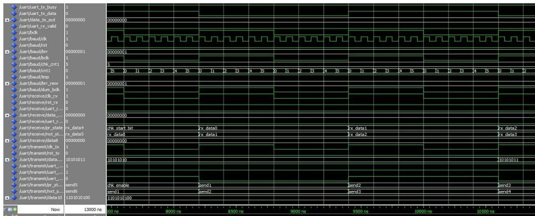
Fig 8 simulation result of fixed baudrate
