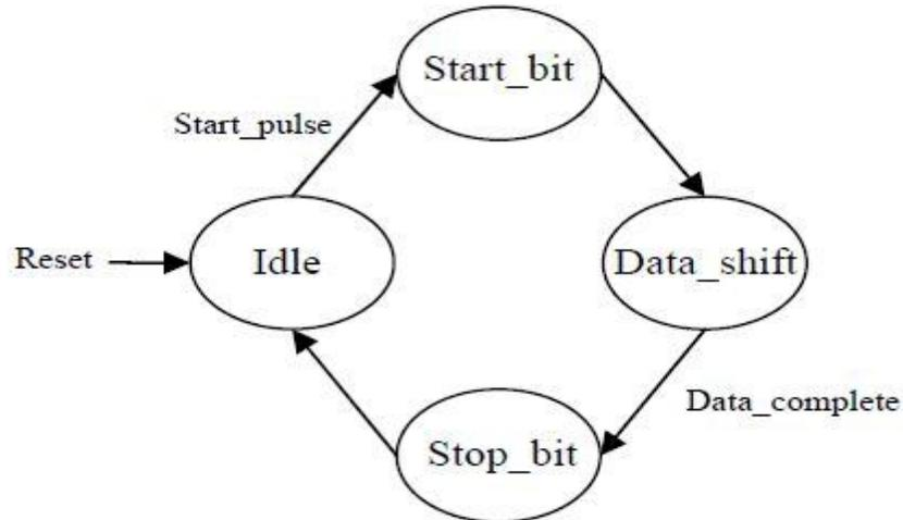
Figure 3 State diagram of a transmitter unit.
