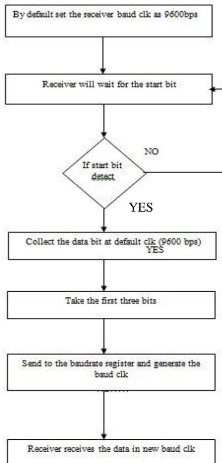
Figure 5 :Flow chart for automatic detection
