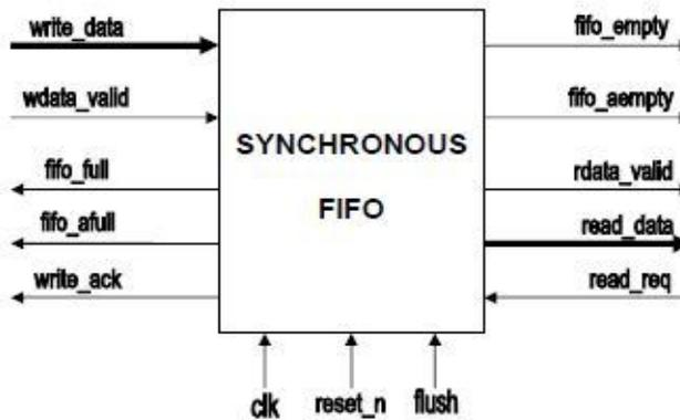
Figure 2: Black-box view of a Synchronous FIFO
