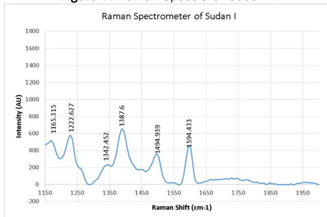
Figure 7 shows Sudan I Raman spectra, characteristic peaks of Sudan dye at 1222.6 cm<sup>-1</sup> represents C-O stretching vibration and CCH scissoring bending of the naphthalene ring, peak 1387.6 cm<sup>-1</sup> is for C=N stretching vibration and C-H in plane bending, Raman peak at 1494.9 cm<sup>-1</sup> displays C=N, N-N stretching vibration, and N-H in-plane bending vibration, and peak at 1594.4 cm<sup>-1</sup> shows C-C scissoring.
