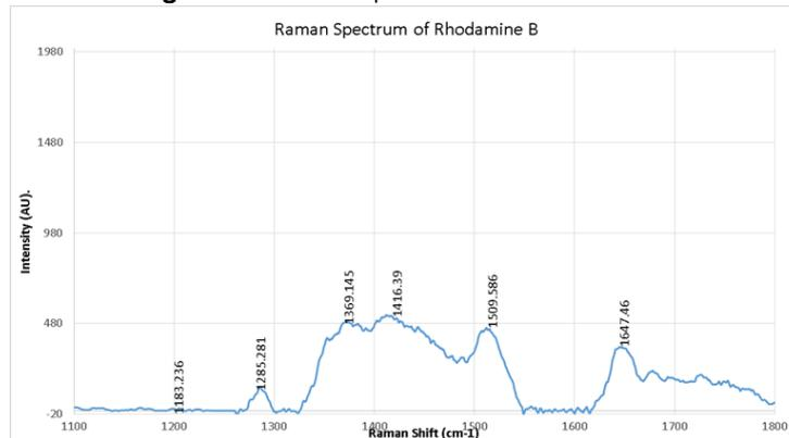
Figure 8 displays Raman spectra of Rhodamine B produces characteristic peaks located at 1183.2 cm<sup>-1</sup> (CH bending), 1285.2 cm<sup>-1</sup> (methyl wagging), 1369.3 cm<sup>-1</sup> (XR stretching), 1509.5 cm<sup>-1</sup> (XR stretching), and 1647.46 cm<sup>-1</sup> (XR stretching) (Figure 9).
