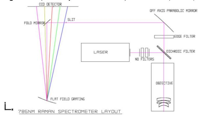
Slit determines the Resolution of the spectrometer but compromise the intensity of light. When slit size is more, less intensity of light observed and resolution gets increased, vice versa. A slit of 50 micron from Thorlabs is used in Raman spectrograph design.
