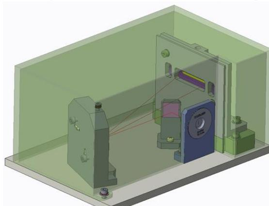
Figure 6. Optical layout of Raman spectrometer (Zemax).
