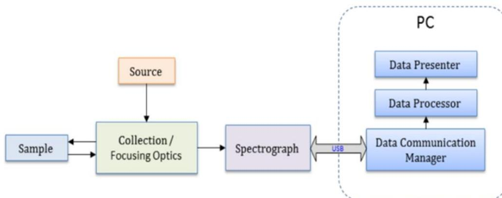
Figure 4B. Raman spectrometers layout.
