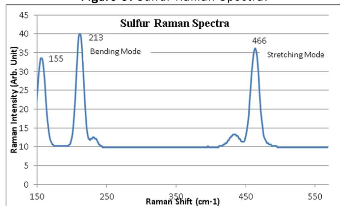
Sulfur spectra shown in Figure 9 in of Cyclo S8 sulfur. It gives 156 cm<sup>-1</sup>, 210 cm<sup>-1</sup> corresponding to sulfur bending mode and peak at 464 cm<sup>-1</sup> shows stretching mode of vibration. Further these spectral peaks can be stored in the data base and software/application can be developed with noise cancellation algorithm to state about the sample directly.
