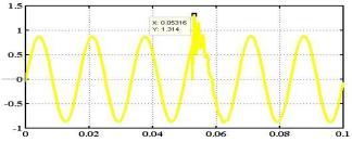
Fig. 10. Voltage Transient which is 130% of its Normal Steady State Value
