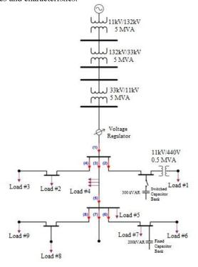
Fig. 1. Radial Feeder System-13 bus system
