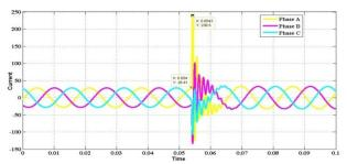
Fig. 4. Inrush Current Observed Near the Capacitor Bank
