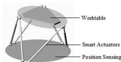
Figure 4: Adaptive Worktable with motion Control System
