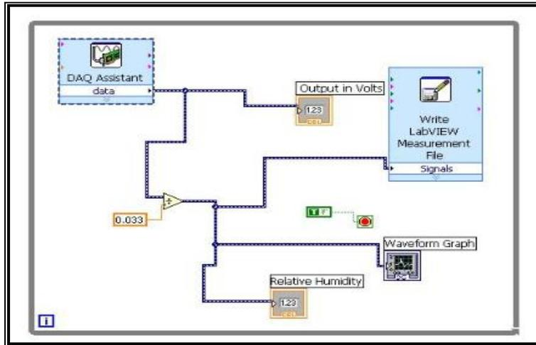
Fig 2(a): VI Block diagram of Humidity Measurement
