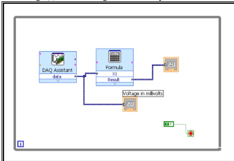
Fig 2(b): VI Block Diagram of Temperature Measurement
