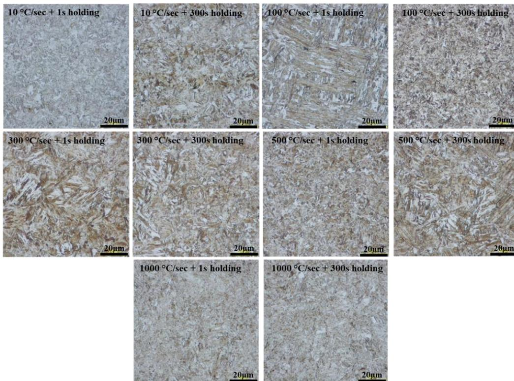
**Figure 7.** The SEM microstructure (at 10000 x) of the steel heated at heating rates 10°C/s, 100°C/s, 300°C/s, 500°C/s and 1000°C/s. and hold at 1 second and 300 seconds. Where  $\alpha$ - Ferrite;  $\alpha'$ -martensite;  $\alpha B$ -Bainite.
