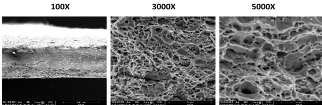
**Figure 9.** Fractograph image at necked region after tensile test the steel heated at heating rates 10 °C/s, 300 °C/s, 500 °C/s and 1000 °C/s. and hold at 1 second and 10 °C/s, 300 °C/s of 300 seconds.
