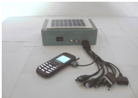
Fig. 1 Charging Li-Ion battery of mobile phone by portable solar charger
