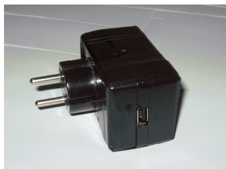
Fig. 6 Voltage source of 5 V with USB connector on its output
