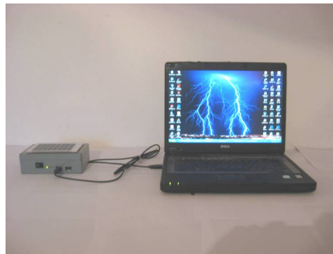
Fig. 2 Charging of NiMH batteries inside portable solar charger by computer through USB port
