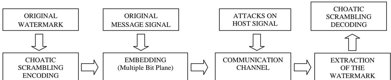
Figure 1. Basic Model of Watermarking
