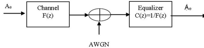
Figure 7: Zero Forcing Equalizer.
