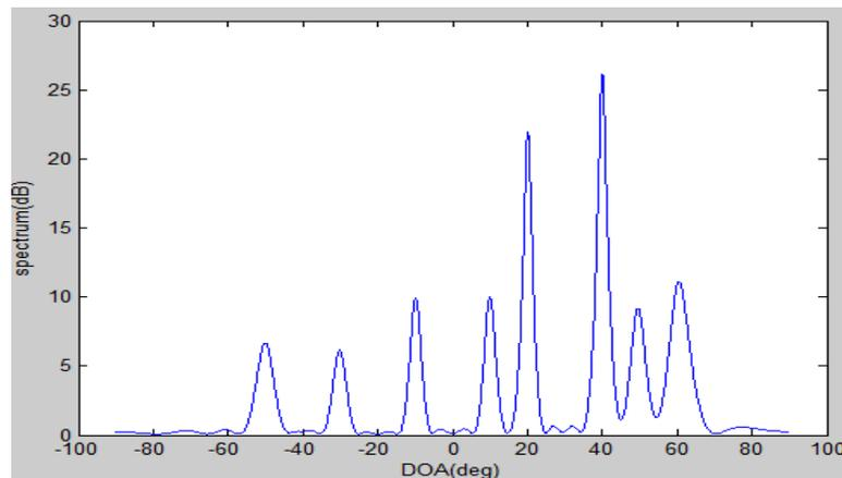
Figure 1: Array pattern of received signal
