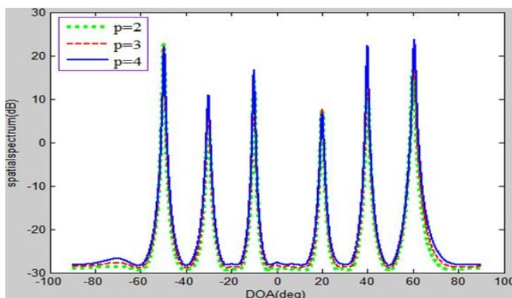
Figure 7: Array pattern versus the less number of sub arrays
